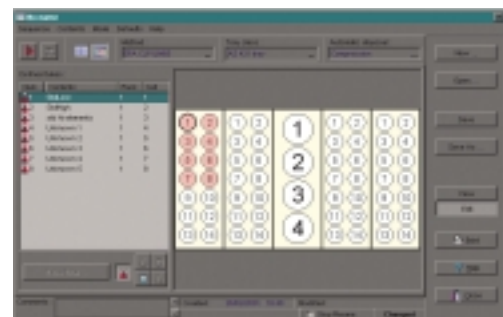
Autosampler locations can be defined using drag-and-drop. Several standard racks exist and custom racks and tube sizes can easily be created using the flexible Analyst software.
