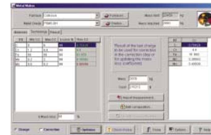
▲ Metal Maker provides automatic charge calculation and exact assistance for the manufacture of accurate alloys based on a defined composition.
