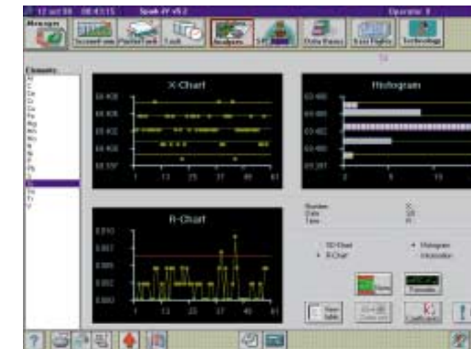
▲ Statistical Process Control (SPC) allows control of the entire process through to production and is useful for the verification of instrument performance.
